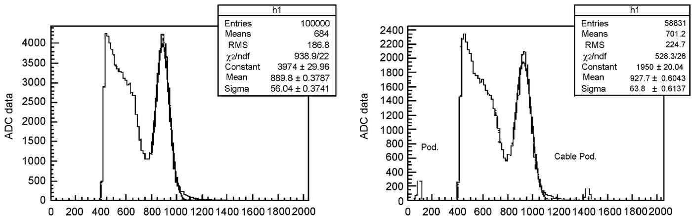
Fig. 4. Comparison of <sup>137</sup>Cs gamma ray spectra taken with the RatCAP chip inside and outside the 4 T magnetic field of the MRI.
